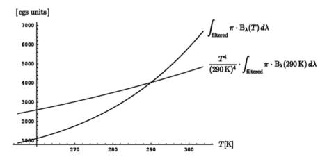
Fig. 4. Black body radiation compared to the wradiation of a sample colored body. The nonuniversal constant  $\sigma$  is normalized in such a way that both curves coincide at T=290 K. The Stefan–Boltzmann  $T^4$  law does no longer hold in the latter case, where only two bands are integrated over, namely that of visible light and of infrared radiation from 3  $\mu$ m to 5  $\mu$ m, giving rise to a steeper curve.
