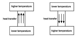
Fig. 31. Any machine which transfers heat from a low temperature reservoir to a high temperature reservoir without external work applied cannot exist: A *perpetuum mobile of the second kind* is impossible.
