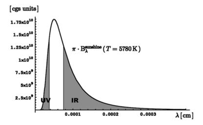
Fig. 5. The spectrum of the sunlight assuming the Sun is a black body at  $T=5780~\mathrm{K}$ .
