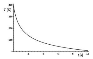
Fig. 27. The cooling curve for a radiating standard cube.
