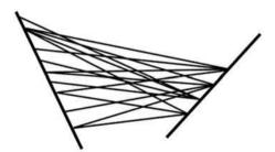
Fig. 3. The geometry of classical radiation: Two surfaces radiating against each other.
