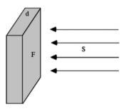
Fig. 14. A solid parallelepiped of thickness d and cross section F subject to solar radiation.
