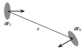
Fig. 1. The geometry of classical radiation: A radiating infinitesimal area  $d\mathbf{F}_1$  and an illuminated infinitesimal area  $d\mathbf{F}_2$  at distance  $\mathbf{r}$ .
