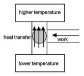
A heat pump (e.g., a refrigerator) works because an external work is applied.
