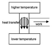
A steam engine works transforming heat into mechanical energy.
